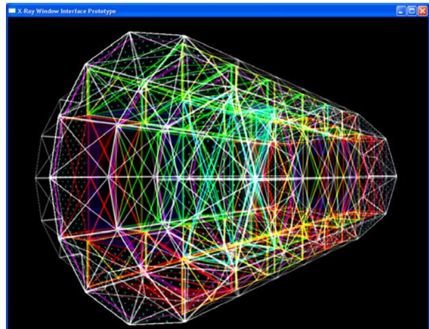
Figure 1. X-Ray Window Rendering of ISS *Destiny* Module, with Color-Coded Stowage and Equipment Components
