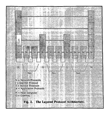
capable of delivering packets from source to destination. At the next layer, end-to-end communication services are built in, including mechanisms such as end-to-end reliability and network control. Finally, at the upper layer, applications services are provided such as file transfer, virtual terminal, and mail.
