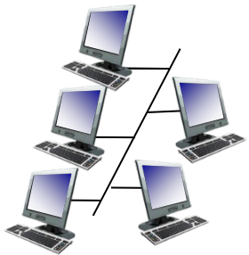
shared wire (e.g., cabled Ethernet)
