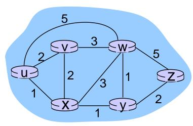
clearly,  $d_{v}(z) = 5$ ,  $d_{x}(z) = 3$ ,  $d_{w}(z) = 3$ B-F equation says:  $d_{ii}(z) = \min \{ c(u,v) + d_{ii}(z), i \}$  $c(u,x) + d_x(z),$  $C(u,w) + d_w(z)$  $= \min \{2 + 5,$ 1 + 3, 5 + 3 = 4 node achieving minimum is next hop in shortest path, used in forwarding table
