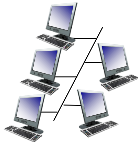
shared wire (e.g., cabled Ethernet)
