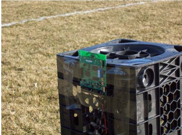
Figure 3d Close view of the receiver: MCF5208EVB with battery power supply
